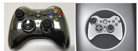
Object: Embossed Logo on Metallic Surface Dome light removes the glare and provides a high contrast image.
