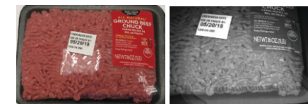
Object: Plastic Food Packaging Wash down dome light allows a clear image showing
