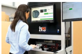
Object: Optical Inspection of PCB board Machine reads the component's datamatrix serial number and checks the part's body for surface defects.
