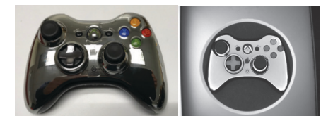
Object: Embossed Logo on Metallic Surface Dome light removes the glare and provides a high contrast image.
